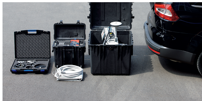
From left to right: Optional Wheel Sensor, battery with power cable and rain cover, sensor system.
